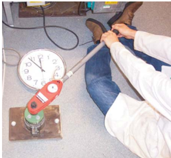
Figure 4.12. Manual torque bond test in progress
