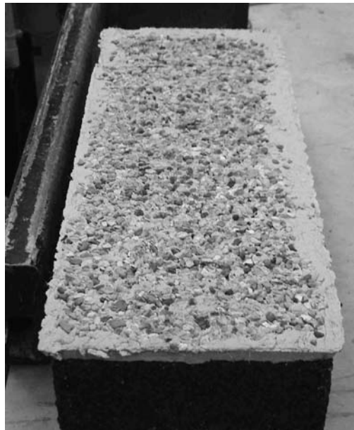
Figure 5.20. Typical sandwich samples of HPCM cast over an asphalt concrete prism
