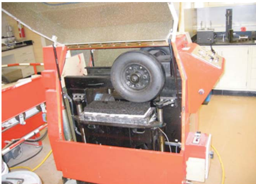
Figure 4.17. Composite Testing of Slab using the French Wheel Track Test
