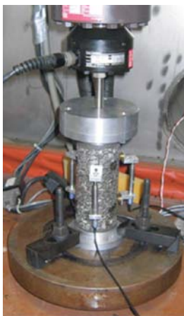
Figure A5.5. Push-Pull Axial Fatigue Set-up
