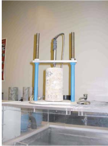
Figure 5.4. CTE frame and LVDT dilatometer device
