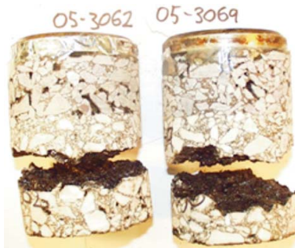
Figure 4.13. Appearance of torque test failure plane SMA (Epoxy) on DBM (100/150pen)
