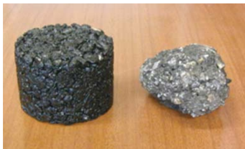
Figure 4.19. Mix Specimens Before (left) and After (right) the Cantabro Test
