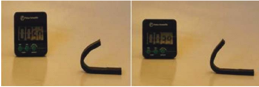
Figure 4.3. Demonstration of Memory Effects in Epoxy Asphalt
