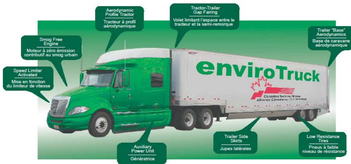
Figure 5.13. The Canadian “EnviroTruck” concept (2007) with fuel-reducing improvements
