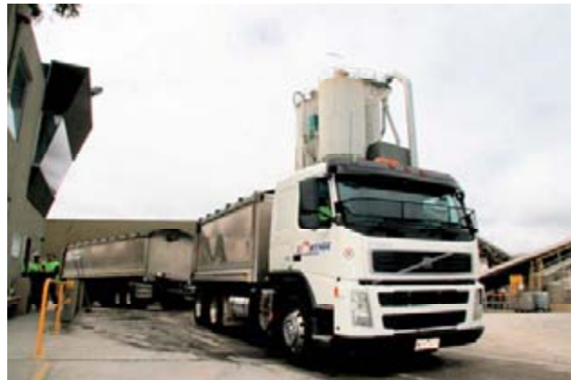
Figure 9.1. PBS case study: high payload truck-trailer for quarry operations
