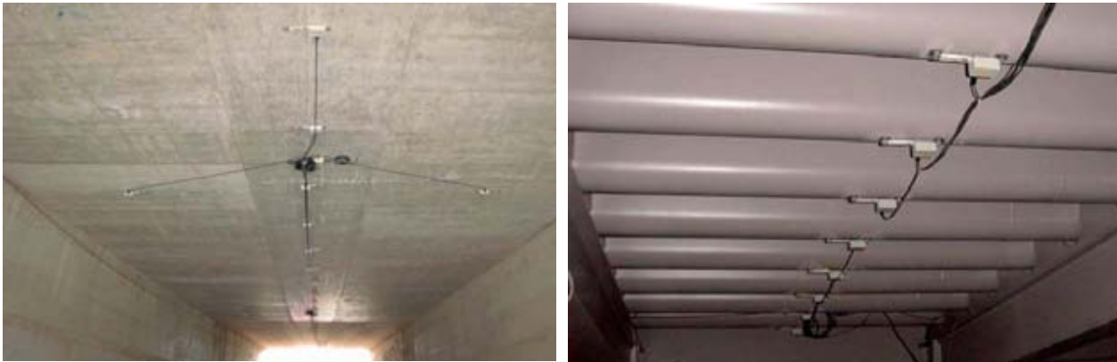
Figure 7.19. Strain measurements with a bridge WIM system on a concrete slab bridge (left) and on an orthotropic deck (right)
