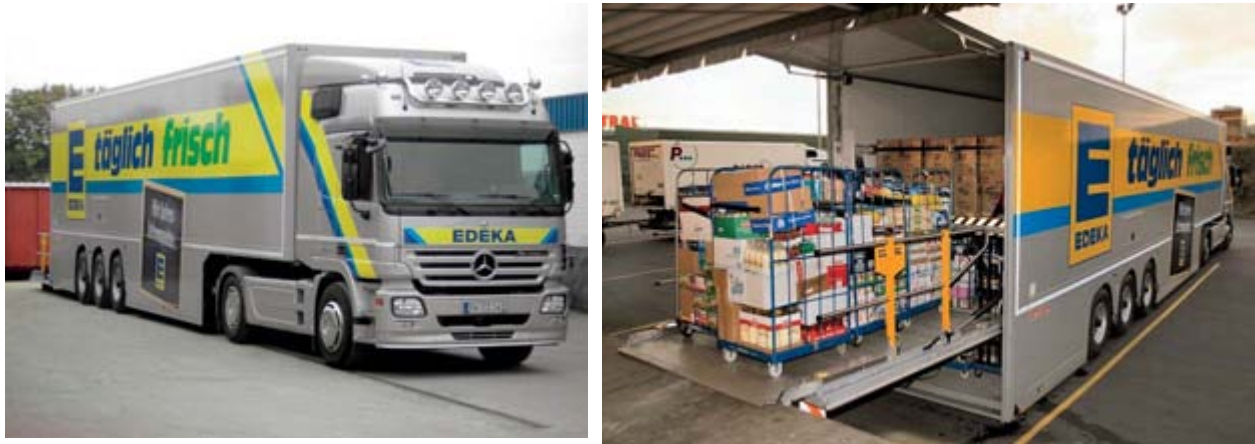
Figure 2.1. Two floor semitrailer with lift, 40 cm ground clearance and 4 m box height, length 16.50 m, single-wheel suspension on semitrailer for volume transports
