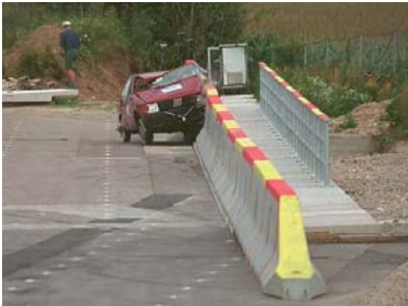
Figure 7.20. Example for impact tests TB 11 (left) and TB 81 (right) on a safety barrier for bridges
