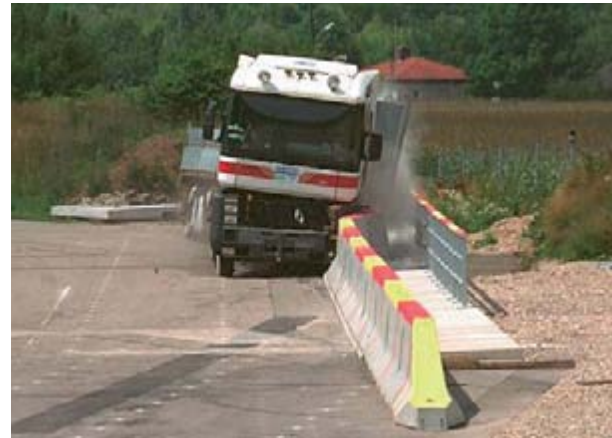
Figure 7.20. Example for impact tests TB 11 (left) and TB 81 (right) on a safety barrier for bridges
