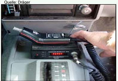
If the BrAC is over a defined threshold, the vehicle cannot be started
