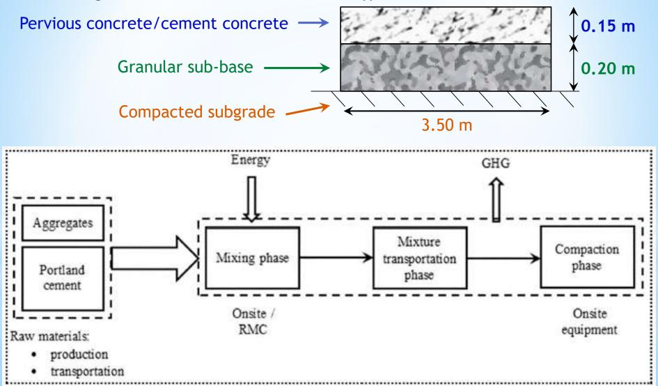
Lifecycle phase and components within system boundary for different pavement systems
