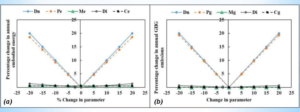
Sensitivity of density, production, mixing, compaction, and transportation distance for: (a) Embodied energy; (b) GHG emissions
