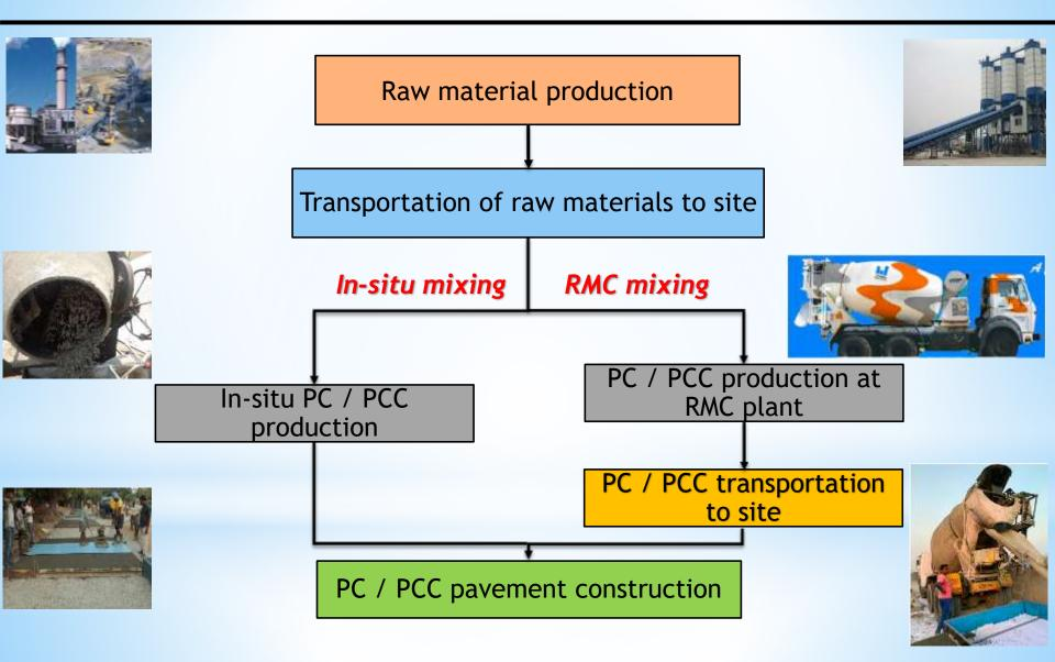
PC - Pervious concrete; PCC - Portland cement concrete; RMC - Ready mixed concrete
