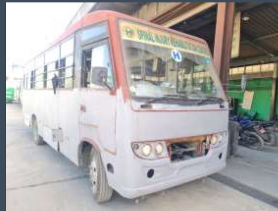
Solutions Plus supported Sajha Yatayat (2024) – converting Nepal's first 6-wheeler – a 26-seater bus – Completed now – Looking for FIRST in NEPAL Approval and Registration
